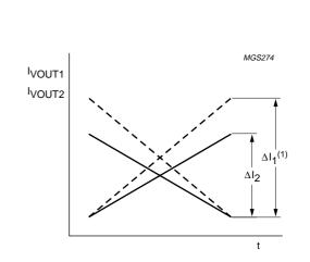
(1)  $\Delta I_1$  is the maximum amplitude setting at register VSIZE = 127, register VGAIN = 63, control bit VOVSCN = 0.
