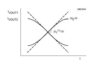
(1)  $\Delta I_1$  is the maximum amplitude setting at register VSIZE = 127 and VLIN = 0%.
