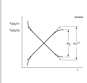
(1)  $\Delta I_1$  is the maximum amplitude setting at register VSIZE = 127 and register VOVSCN = 0.
