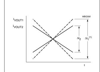
(1)  $\Delta I_1$  is the maximum amplitude setting at register VSIZE = 127, register VGAIN = 63, control bit VOVSCN = 0.
