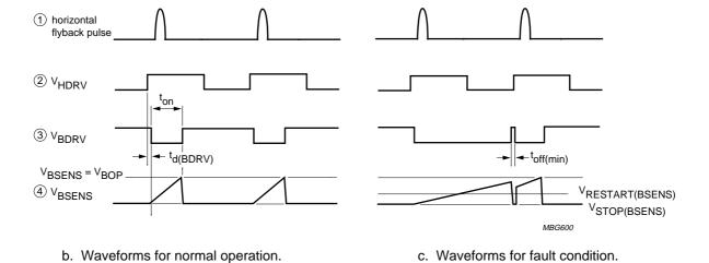
Fig.22 Application and timing for feedback mode.
