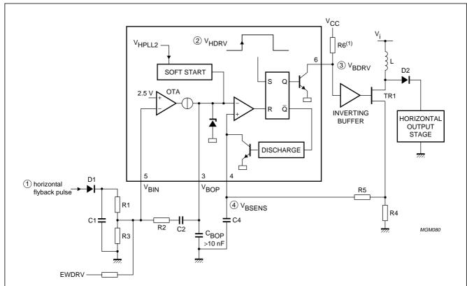
For f < 50 kHz and C2 < 47 nF calculation formulas and behaviour of the OTA are the same as for an OP. An exception is the limited output current at BOP (pin 3). See Chapter "Characteristics", Row Head "B+ control section; see Figs 22 and 23".
